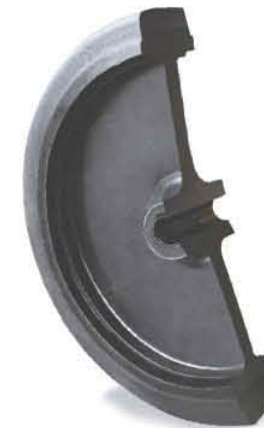
301B BLACK TREAD Temperature Range: -10°F~150°F Hardness: 75±5 shore A
